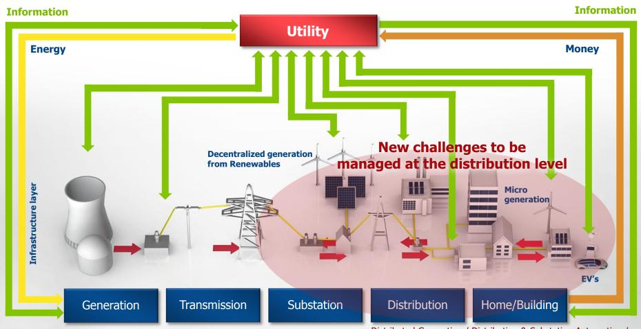
Distributed Generation / Distribution & Substation Automation / Dynamic Load Management / Dynamic Tariffs / Local Load Controller (Micro Generation) / EV's / New Energy Services / Personal Energy Mamt
