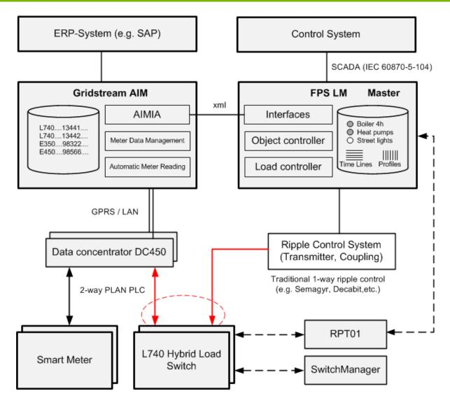
L7XX: Modern 2-way PLAN PLC AND traditional 1-way ripple control communication within ONE system
