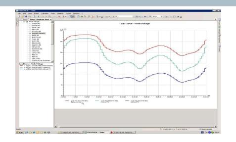
The network simulation gives you results for the loading of the network and for the voltage ranges during the day in every location
