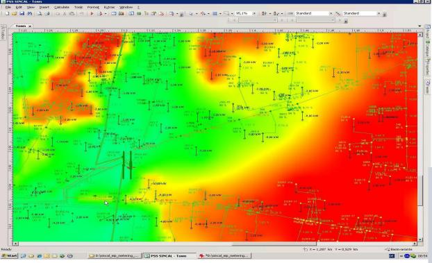
With a suitable network configuration a change of parts of a feeder to an adjacent feeder can optimize generation and losses in the network
